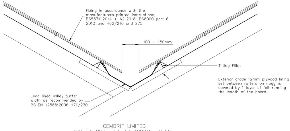
VALLEY GUTTER LEAD TYPICAL DETAIL 508x254 GLENDYNE (NATURAL SLATE) DRG No. 570 H62/105, 280 and 615
